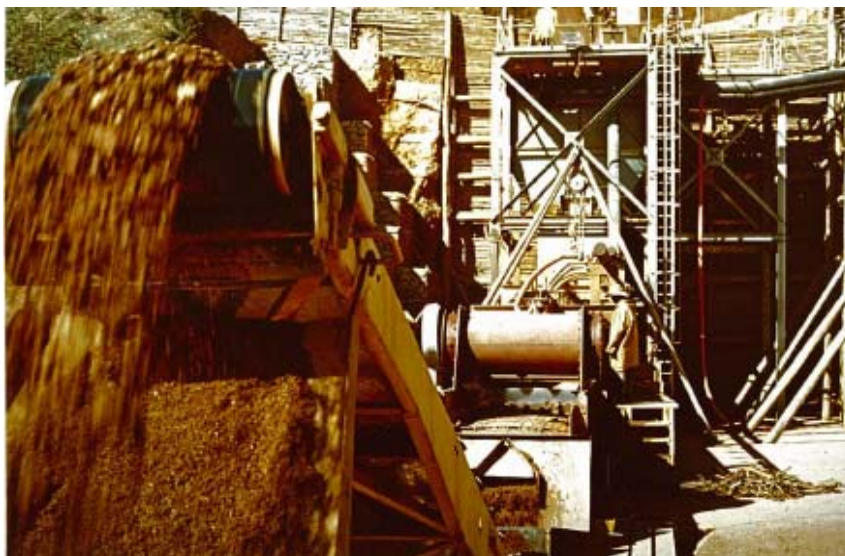
Figure 5.1. Washing pilot unit.
